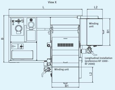
Transverse installation (KF 1000 - KF 2000) Only separate transport possible
